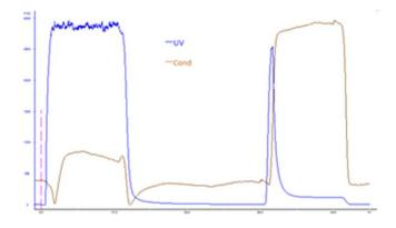
Column: EzFast 1mL Bed height: 2.5cm Buffer solution: A: 25mM imidazole + 0.15m NaCl pH: 7.00 B: 500mM imidazole pH: 7.00 Sample: *E.coli* expression was recombinant with His-GST label Loading quantity of sample: Supernatant of protein lysate 10mL Flow velocity: 1mL/min
