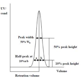
As a guideline, if the value of HETP is less than 3 times the average particle  $size(d_{50})$  of the resin and the As is between  $0.8\sim1.8$ , the column is very efficient. The unsatisfactory results should be analyzed and the column should be repacked.
