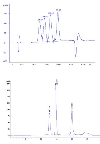
Column: BXR10/17 Mobile phase A: 0.1% trifluoroacetic acid+water Mobile phase B: 60.0% acetonitrile, 0.1% trifluoroacetic acid+water Samples: Angiotensin I, Angiotensin III, (Val<sup>4</sup>) Angiotensin III, (Ile<sup>7</sup>) Angiotensin III
