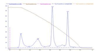
Column: BXR 10/17 Equilibration: 20mM Tris 1.7M (NH<sub>4</sub>)<sub>2</sub>SO<sub>4</sub> pH 7.5 Elution: 20mM Tris pH 7.5 Sample: Cytochrome C 1 mg/mL Lysozyme 1mg/mL RNA enzyme 2mg/m α-Chymotrypsinogen1mg/mL
