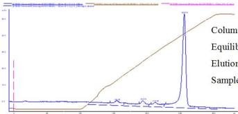
Column: EzScreen 4.2mL Equilibrium buffer:20Mm HCOOH pH 4.0 Elution buffer : 20mM HCOOH +0.75M LiCl pH 4.0 Sample: WGA and β -lactoglobulin mixture
