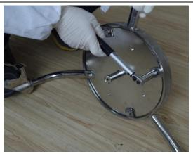
d. Place the support net plate flat in the center of the end-piece.
