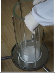
c. Buckle the upper O-ring into the flange.
