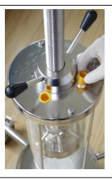
c. Before use, tighten the nut of feed port to avoid the risk of leakage (if the sealing ring of feed port is damaged, it needs to be replaced in time). If external pipe connection is
