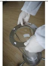
e. Put in the gasket and tighten with a torque wrench.
