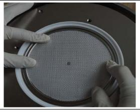
f . Install the lower O-ring between the guide ring and the lower net.
