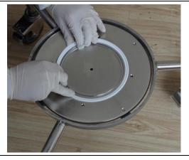
e. Install the lower filter net.
