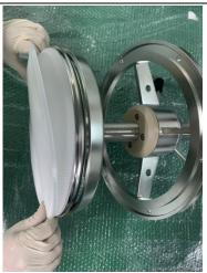
b. Install the installed adapter into the glass tube
