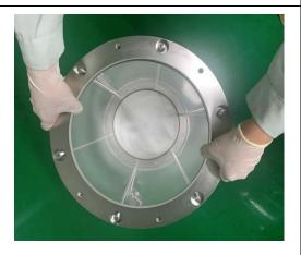
e. Put in the gasket and tighten with a torque wrench.
