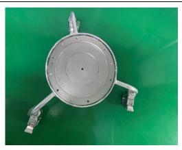
c. Place the guide plate face up in the middle of the chassis and clamp it into the chassis groove. Then place the lower support net evenly in the center of the chassis and clamp the lower screen net in the outer ring groove of the chassis.
