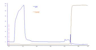
Column: EzScreen4.4mL Buffer A: PBS pH7.5 Buffer B: 1M NaOH+1M NaCl Sample: virus Flow velocity: 0.6mL/min
