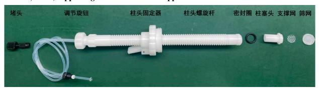
• Lower adaptor consists of plug, soft pipe, bottom rod, adjusting knob, adaptor fastener, O-ring, sieve, supporting sieve and column stopper.
