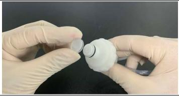
g. screw bottom fastener to the column bottom
