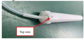
When mounting/removing adaptor, the O-ring should be loosen. If O-ring blocks, gently switch the adaptor. Never push/pull violently or shake adaptor to avoid breakage in glass tube.
