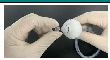
f. Fasten the sieve on the column stopper
