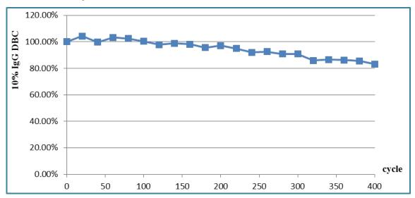
AT Protein A Diamond plus with 0.1M NaOH CIP (residence time: 15min) for 10%IgG dynamic load
