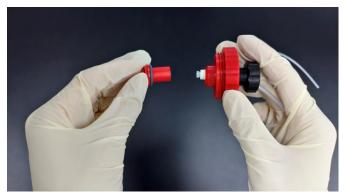
e.Place the supporting mesh on the column stopper
