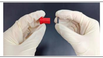
d.Connect the column stopper (with O-ring)to screw rod, tighten it(make sure gasket and hose are properly connected before assembling)
