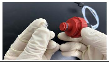
f. Buckle the sieving mesh on the column stopper
