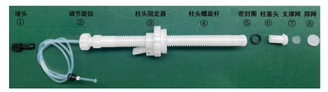
Note: ①plug②adjusting knob③cylinder head fixer④cylinder head screw rod
