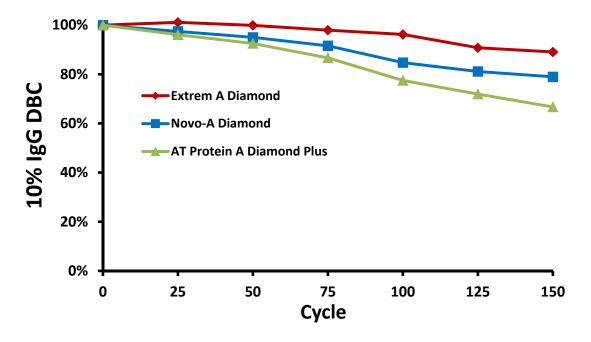
10% IgG DBC variation after using 0.5M NaOH for CIP (Residence time 15min)
